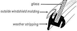
**3.** Apply a continuous bead of sealer to the windshield opening flange on the car. Apply a continuous bead of sealer into the glass crevice of the rubber seal then install the weather strip onto the glass. If the car also has outside windshield moldings, they must be installed into the weather stripping at this time.
