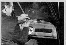
Remove gamish moulding screws carefully and prepare to cover dash with masking tape and protective material
