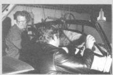
With two pair of hands, carefully insert complete windshield unit from interior
