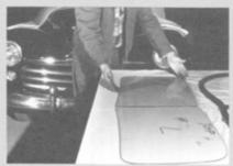
Mark windshield right and left with grease pencil. Note bottom curvature on both glass pieces.
