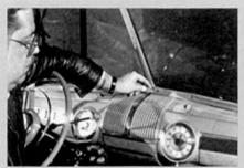
Plastic wiper knob pulls off. Nut must be removed to release switch to underside of dash.
