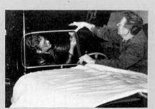
While removing center post screws, have one person hold exterior center strip to prevent falling on hood.
