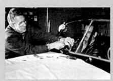
With sharp knile, carefully cut exterior weathershipping away from glass.
