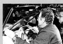
With two pair of hands, carefully allow windshield to drop down and out to interior of the car.
