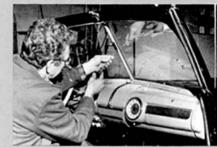
Begin by removing windshield wipers and rear view mirror.
