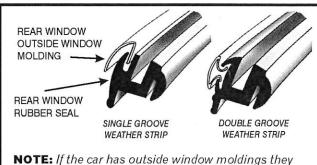
**NOTE:** If the car has outside window moldings they must be installed into the weather stripping at this time. Two types of rubber seals were used: Single groove and double groove.
