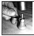
To install the knob to the handle, place the knob face down on firm surface such as a book. Position the handle and insert the pin through the handle and into the knob. Lightly tap the pin into the knob with a hammer. Use a punch to set the pin deeper into the handle but leave enough play to allow the knob to rotate.
