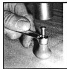
To install the knob to the handle, place the knob face down on firm surface such as a book. Position the handle and insert the pin through the handle and into the knob. Lightly tap the pin into the knob with a hammer. Use a punch to set the pin deeper into the handle but leave enough play to allow the knob to rotate.
