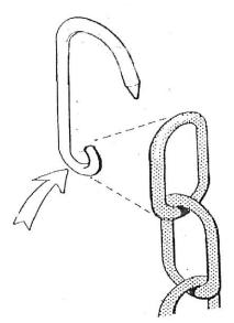
1. Open the "eye" end of the hook, insert the welded chain link end and close the eye tightly.
