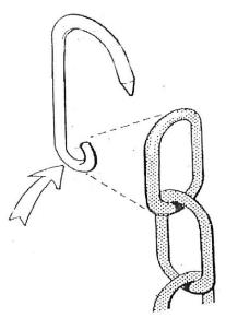
1. Open the "eye" end of the hook, insert the welded chain link end and close the eye tightly.
