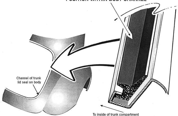
Use weather stripping adhesive (#COAZ-19554-A) to secure trunk seal into channel
