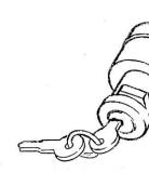
To work properly, run a ground wire from ground terminal to engine or frame. Install switch so terminals do not touch inner support bracket on shroud.
