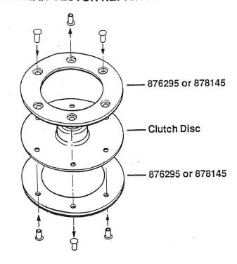
AND ALIGN THE MATCHING HOLES SO THE SIX (6) RIVETS CAN BE INSERTED.
