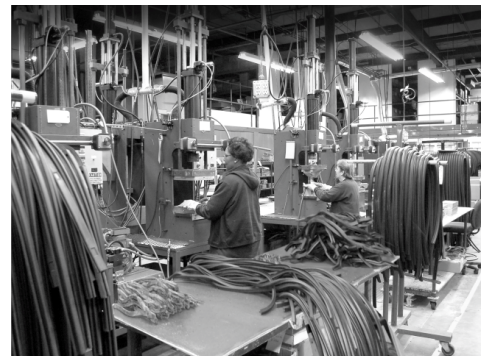
The rubber molding department is responsible for final assembly of door and trunk seals.
