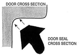
Door seal lays in the corner all the way around the door.
