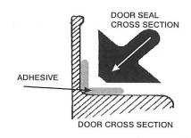
NOTE: It is necessary to use a weather stripping adhesive in order to install door seals. Dennis Carpenter Ford Reproductions recommends and sells 3M brand Weather Stripping Adhesive. Our part # is COAZ-19554-A
