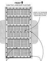
KNURLED BOLTS AND NUTS WITH LOCK WASHERS AND SMALL FLAT WASHERS (Knurled bolts used on the bed strips only)
