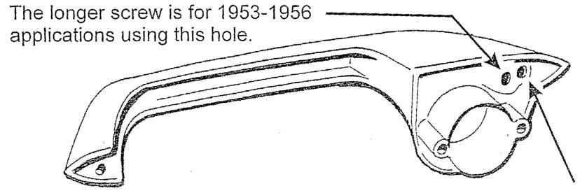
The shorter screw is for 1957-1960 applications using this hole.
