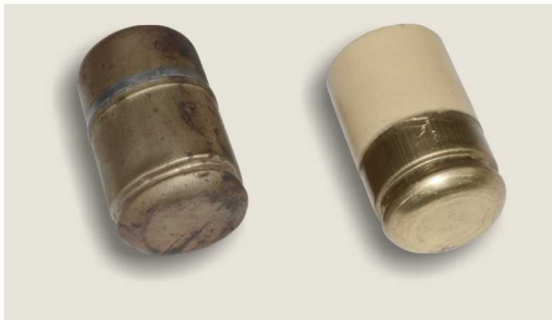
Original brass floats (left) were prone to leakage after time and would sink. Modern fuel resistant, foam floats never leak thus stay afloat.
