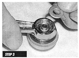
Place knob face down onto a solid protective surface. Push down on the handle to compress the spring and place the washer onto the shaft.
