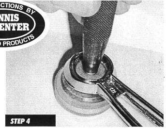
Place a 15/32" center punch into the center of the knob stud. Firmly tap the punch with a hammer to flare out the sidewalls of the knob stud.
