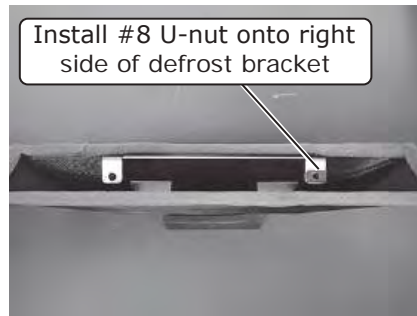
Passenger Side Defrost Duct
