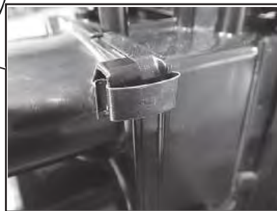
Spring Clip Installed Photo 3
