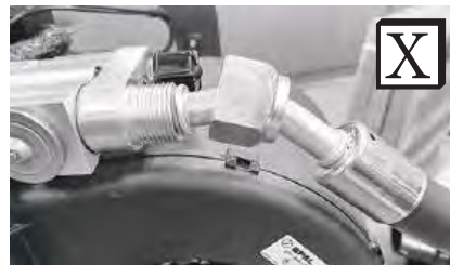
Improperly Seated O-ring Land
