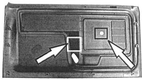
Markings locate holes for factory power door locks and power window switches.
